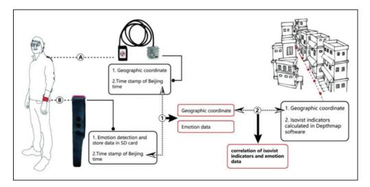
**Figure 2.** Diagram of the portable experimental equipment. Each subject wears a GPS receiver (with active GPS antenna) and a BodyMonitor smart band (that records skin conductivity). Both items record the time stamp of Beijing at the same time, and we therefore assigned the emotional data to the geographic coordinate and built a relationship between emotional data and isovist indicators through the geographic coordinate.
